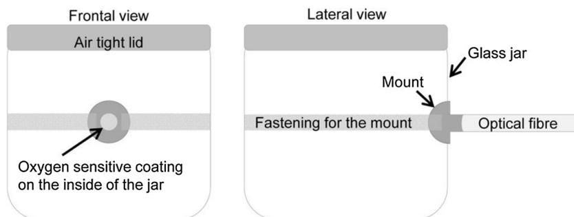
Fig. 3. Schematic overview of the measuring jars used for oxygen consumption measurement.
