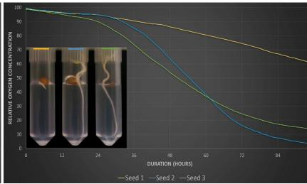
Single seed respiration measurements provide information about differences between seeds in a sample. In this example the germination of three individual seeds in the SRA measuring vials can be seen together with their oxygen consumption profiles. The most vigorous seed (indicated green and green line) is fastest in oxygen consumption, while the least vigorous seed (yellow indicator and line) lags behind in both germination and oxygen consumption.
