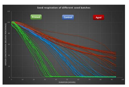
Single seed respiration measurements provide information about differences between seed samples after seed treatments, such as priming and accelerated aging. The example shows that priming (green lines) results in more homogenous (individual seed curves close together) and faster (steeper lines) oxygen consumption as compared to the control seeds (blue lines). Aged seeds (red lines) show reduced and delayed oxygen consumption as compared to control seeds (blue lines).
